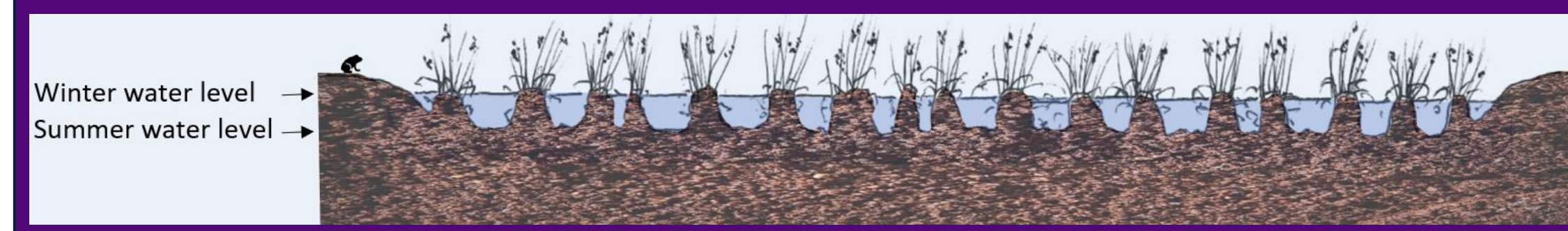
Fig. 6. Scrapes designed to fill up to 30 cm deep in winter and draw down in summer.
