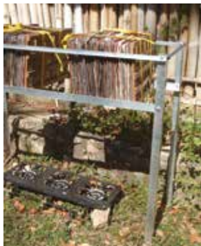
drying frame with gas stove before cover attached
