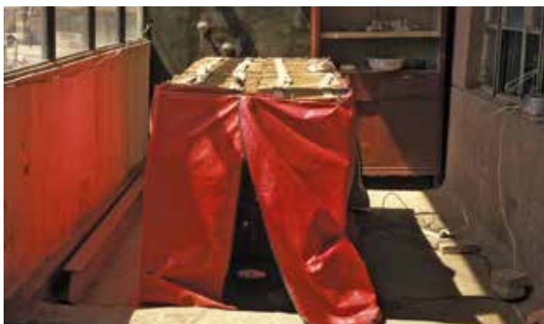
drying frame with electric heaters and cover
