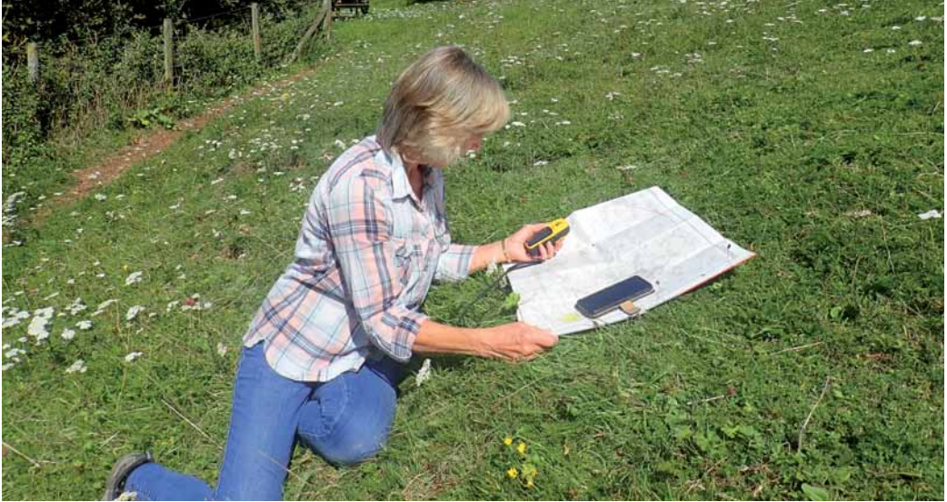
Checking out a grid reference using an OS map and a GPS device. Andrew Branson
